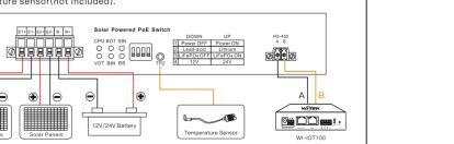
Power Priority: The input priority is determined based on the voltage, and the input
